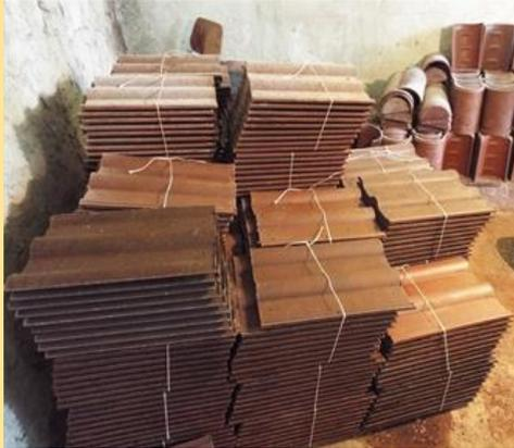
“Levon Avagyan” PE uses plastic waste materials in addition to PE’s annual additional waste processing opportunities. Dilijan based entrepreneurs produce roof tiles (single roof materials typical to Dilijan) made of thick cement mortar and sand mixed with the waste from plastic materials. The production of suggested roof materials containing solar battery elements is one of RECP advanced measures requiring large investments.
