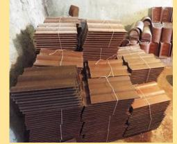
"Levon Avagyan" PE uses plastic waste materials in additional to PE's annual additional waste processing opportunities. Dilijan based entrepreneurs produce roof tiles (single roof materials typical to Dilijan) made of thick cement mortar and sand mixed with the waste from plastic materials. The production of suggested roof materials containing solar battery elements is one of RECP advanced measures requiring large investments.
